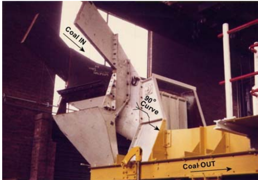
Photograph 2: Spence Chute experiment with 90° curve at Madeley Wood Colliery c1956. Photographs: Ivor Brown
