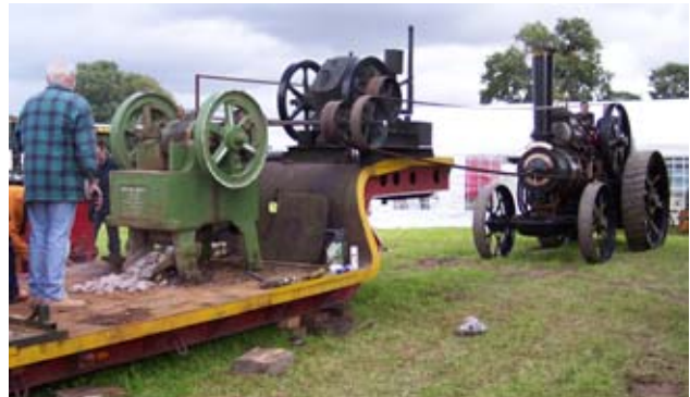
Above: The Fowler traction engine "Pride of the Wye" driving the main crusher.
