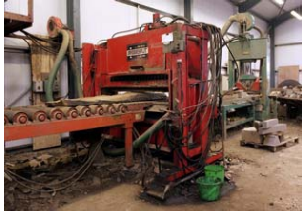
Stone Splitting machine, Flinty Fell Stone Works
