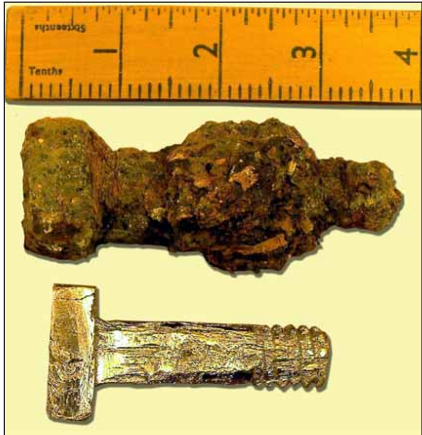
Pitchcroft bolts; before and after polishing. (David Poyner)
