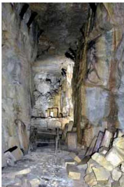
Left & below: Views of a large stone preparation area at the far end of the underground workings. In addition to cutting blocks to shape, it appears banker masons worked here preparing a range of items.
